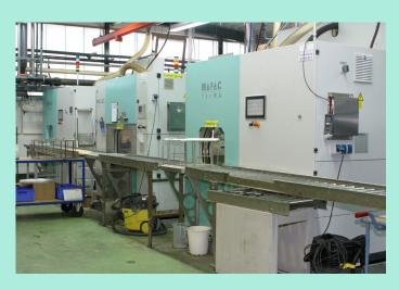
manual roller conveyor was extended by a PALMA with three baths. It is currently used in pre-cleaning. In 2015, another PALMA was installed for final cleaning, as well as another JAVA currently used for drying in final cleaning only.
