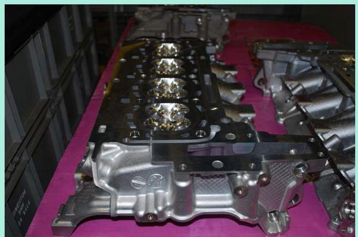
frame. Hidden interior contours and undercuts in the cylinder heads are therefore wetted sufficiently and cleaned thoroughly at a low temperature. In order to relieve stress and pressure, the MAFAC application engineers ensured the cleaning chamber was flooded and emptied quickly, with ultra-fine filters preventing small dirt particles re-contaminating components. Rapid emptying of the cleaning chamber additionally helps to reduce idle time.
