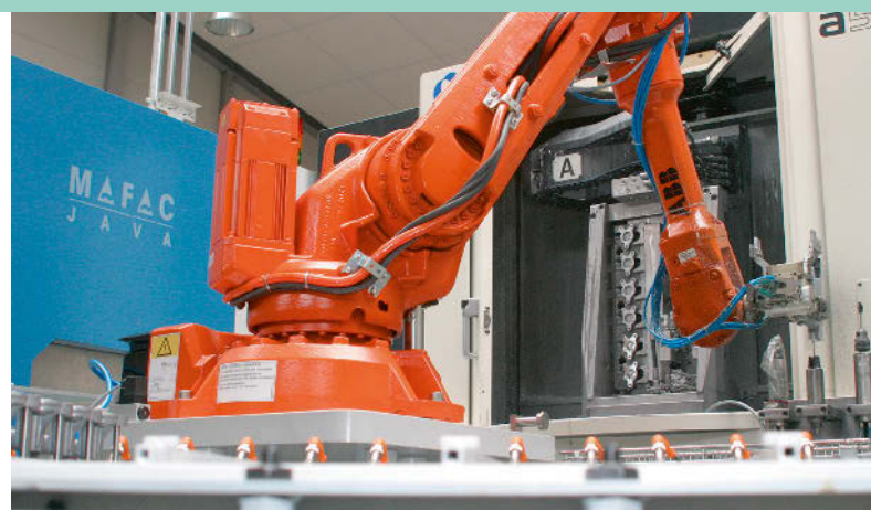
The MAFAC JAVA installed at the Haas premises is fed by a robot which removes the workpieces soiled with emulsion and chips from the adjacent machining centre.
