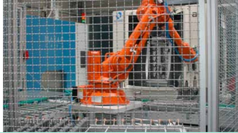
Fully integrated in the automated final assembly of the oil pump housing, the MAFAC cleaning system is installed directly in the robotcell.
