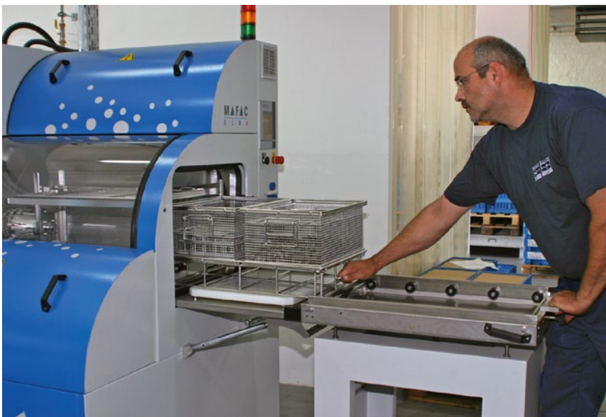
The unit for the second cleaning stage is installed in a separate room and cleans components made of high-alloyed steel and nickel-based material
