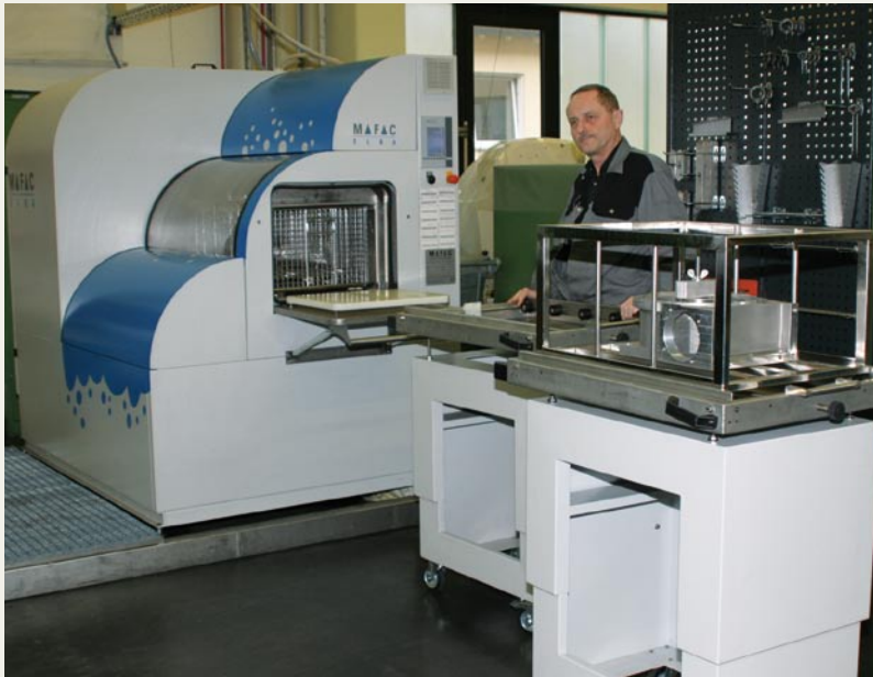
The cleaning machine is an integral part of the assembly line and is installed immediately behind the warehouse.
