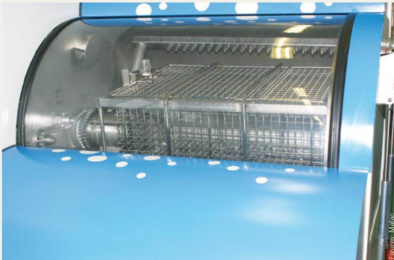
The baskets rotate in the opposite direction to the air jets during the drying process.
